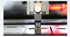
Multiple head configurations allow jetting of different fluids within one process. Up to four Z-axes with valves or placement nozzles can be controlled independently.
