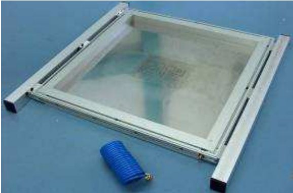
Frame complete with mounted stencil and air tube.
