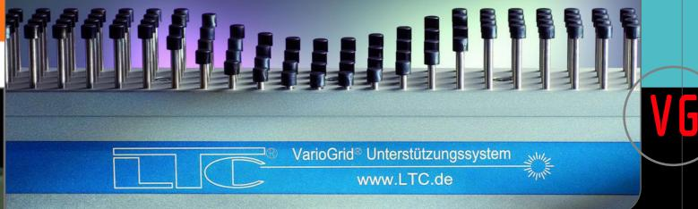
The implementation of the innovative VarioGrid® assembly support system eliminates programming time from individual tooling set-up in printing and placement applications and therefore minimizes common machine down time. The VarioGrid® support system will also eliminate rework due to misplacement of conventional support tools. This results in increased quality as well as throughput and productivity, thus leading to higher cost efficiency for each SMT production line.
